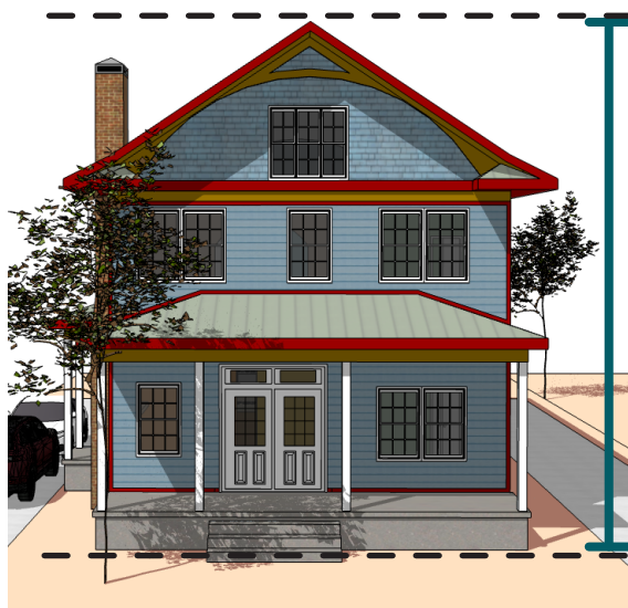
Figure 11: The graphic above shows the height of the structure as the length of the blue line. It spans the distance between the horizontal line at the average grade along the structure's front elevation (lower black dashed line) and highest point of the roof (upper black dashed line).
